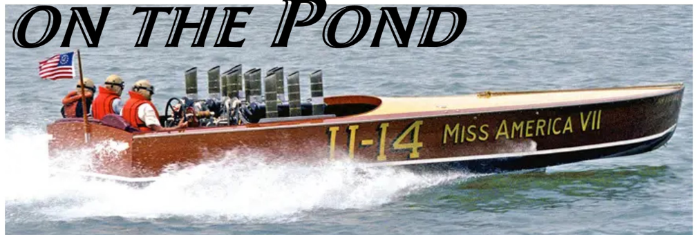
This replica U-4 Miss American VII used a pair of the 1237 engines
